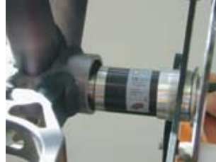
4d. Chain guide: Slide your chain guide and any spacers required (see Chainline Adjustments below) over the spindle assembly.
