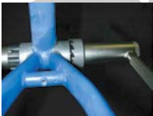
1. Chase and face bottom bracket shell - recommended. This should be performed by a professional bike shop.
