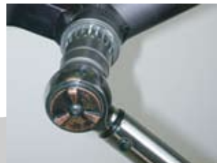
6. Tighten the non-drive side cup until it comes to a dead stop. Check that the cup is torqued to 35 foot-pounds.
