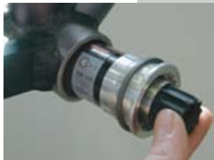
4a. 68mm shell: Slide the included 2.5mm spacer over the spindle assembly so it rests against the flange of the drive side cup.
