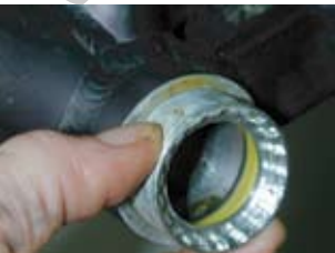
3. Thread the non-drive side cup clockwise three to four turns by hand.
