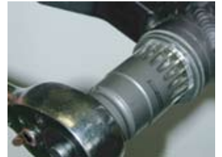
5. Thread the bottom bracket assembly in counter-clockwise and torque drive side cup to 35 ft-lb.
