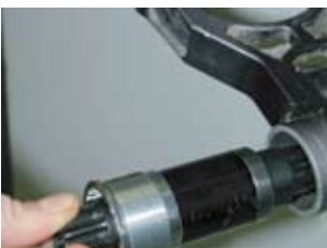
4b. 73mm shell: Do not use the spacer.
