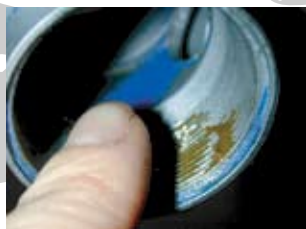
2. Apply a film of grease to the threads inside the BB shell to prevent seizing or galling.
